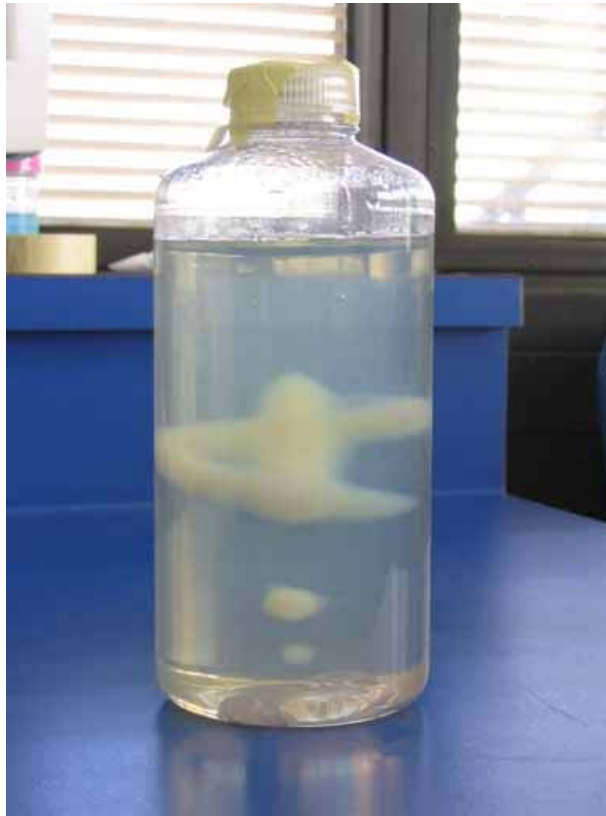
Figure 1: Photograph of a non-uniformly irradiated polymer gel dosimeter.
